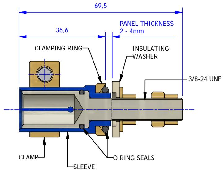
PANEL (BULKHEAD) THICKNESS 2 - 4mm
