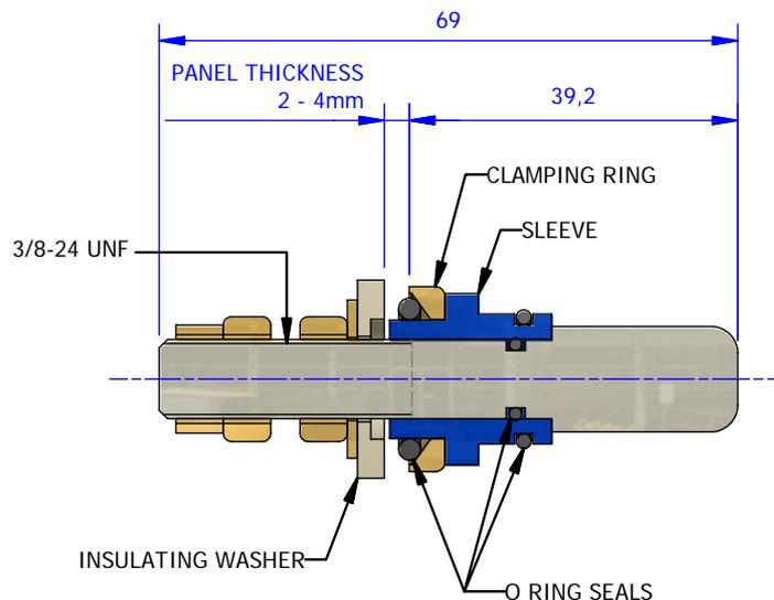
PANEL (BULKHEAD) THICKNESS 2 - 4mm
