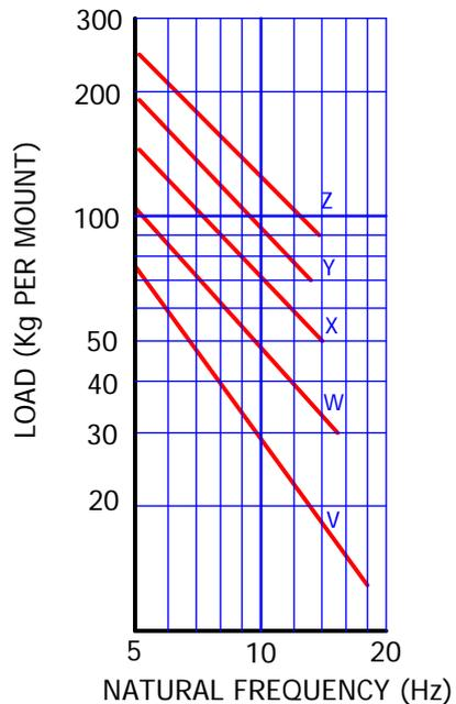
RATING (Kg PER MOUNT =  $\frac{\text{Mass of Unit}}{\text{Number of Mounts}}$ )
